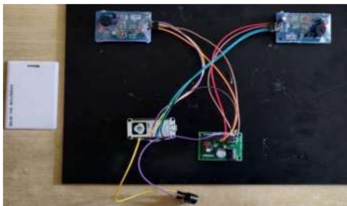
Fig 4: Circuit connection for the RFID prototype
