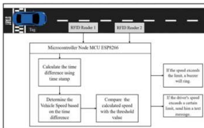
Fig 2: Architecture of the prototype model
